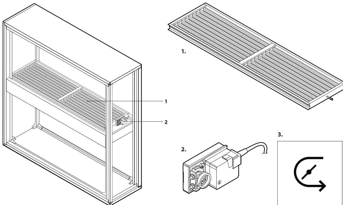
**Fig. 7.** Section recirculation
